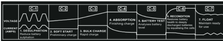
This is a fully automatic battery charger with 7 charging stages.
