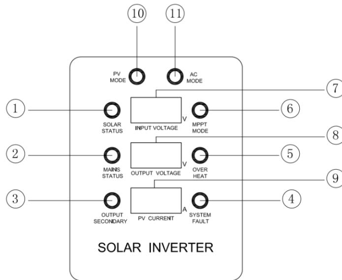
**(1) SOLAR STATUS:** When the SOLAR mode is selected with the button, the LED will light up, and screens (7), (8), and (9) will display PV information.
